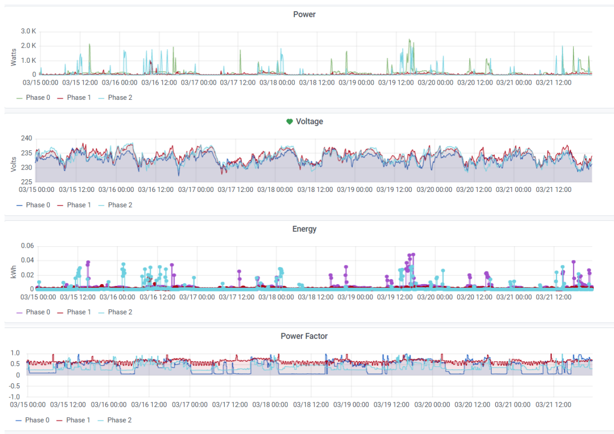
Figure 20 – Historical data for Power, Voltage, Energy and Power Factor per phase
